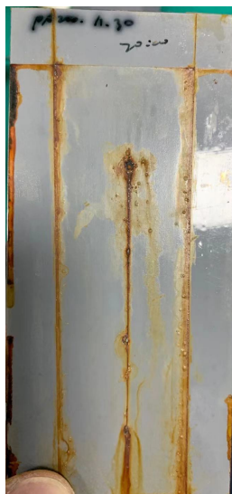
PA200, 1400h盐雾状态 (50 μm, 冷轧钢板)
