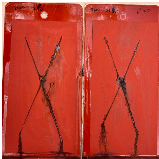
ME3200+MH3939 , 50μm, 冷轧钢板, 盐雾650h 状态
